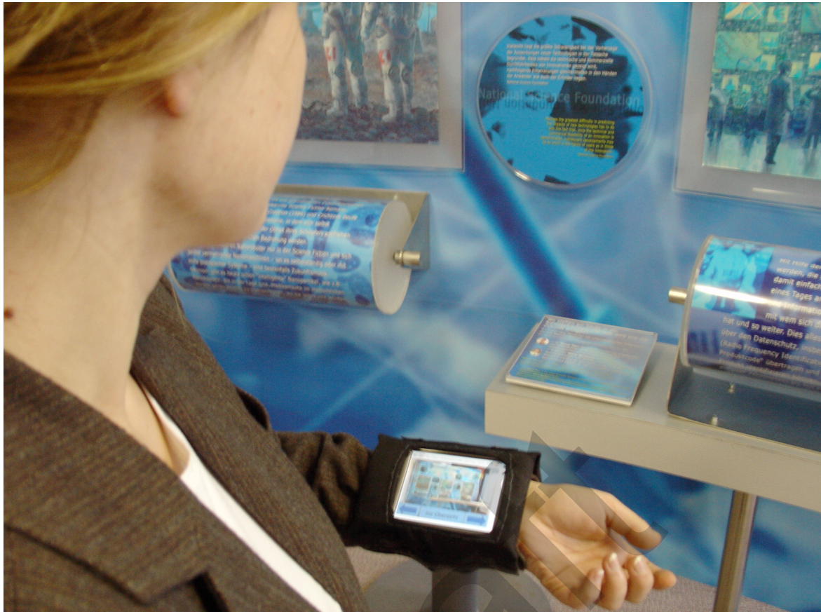
Figure 1: Visitor with PDA – the current exhibition wall is represented on the screen, allowing visitors to select interesting objects to bookmark them or receive more information about them (including access to Wikipedia).
